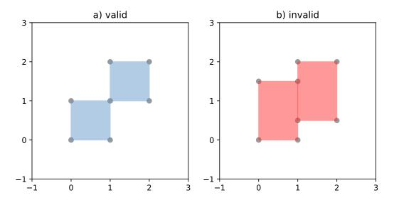
Figure 7. On the left, a valid MultiPolygon with 2 members, and on the right, a MultiPolygon that is invalid because its
