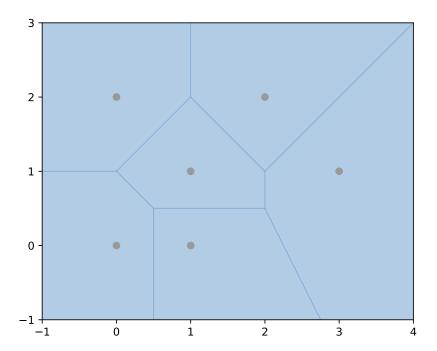
shapely.ops.voronoi\_diagram(geom, envelope=None, tolerance=0.0, edges=False)
