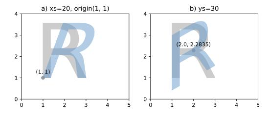
Figure 18. Skewing of a gray "R" to blue result: a) by a shear angle of  $20^{\circ}$  along the x-direction and an origin at (1, 1); b) by a shear angle of  $30^{\circ}$  along the y-direction, using default origin.
