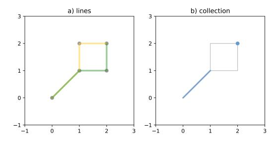
Figure 5. a) a green and a yellow line that intersect along a line and at a single point; b) the intersection (in blue) is a collection containing one *LineString* and one *Point*.
