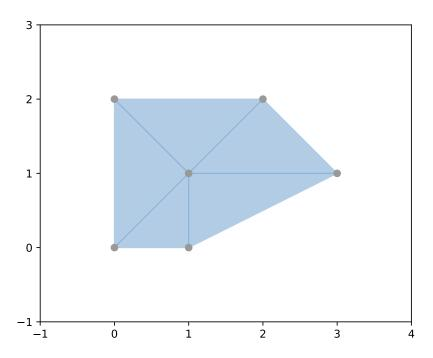
shapely.ops.triangulate(geom, tolerance=0.0, edges=False)
