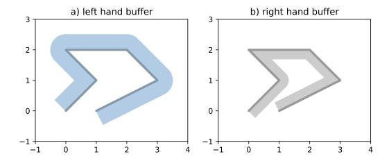
The single-sided buffer of point geometries is the same as the regular buffer. The End Cap Style for single-sided buffers is always ignored, and forced to the equivalent of *CAP\_STYLE.flat*.
