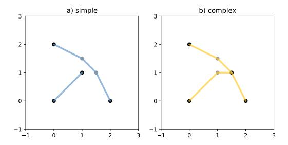
Figure 6. On the left, a *simple*, disconnected *MultiLineString*, and on the right, a non-simple *MultiLineString*. The points defining the objects are shown in gray, the boundaries of the objects in black.
