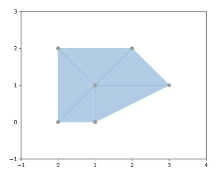
shapely.ops.triangulate(geom, tolerance=0.0, edges=False)
