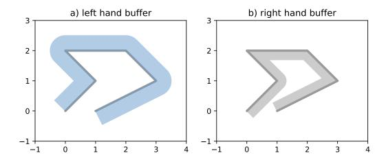
The single-sided buffer of point geometries is the same as the regular buffer. The End Cap Style for single-sided buffers is always ignored, and forced to the equivalent of *CAP\_STYLE.flat*.
