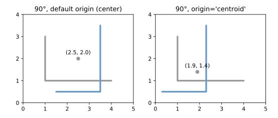
Figure 16. Rotation of a  $\it LineString$  (gray) by an angle of  $90^{\circ}$  counter-clockwise (blue) using different origins.
