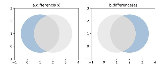
Figure 8. Differences between two approximately circular polygons.
