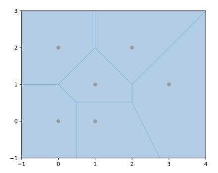
shapely.ops.voronoi\_diagram(geom, envelope=None, tolerance=0.0, edges=False)
