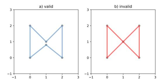
Figure 2. A valid *LinearRing* on the left, an invalid self-touching *LinearRing* on the right. The points that describe the rings are shown in grey. A ring's boundary is *empty*.
